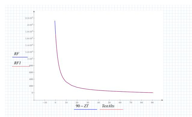
We see that the interpolated points, in red, lie very close to the tabular points, in blue, which was to be expected if the logic of interpolation in procedural function **RFN** is correct.
